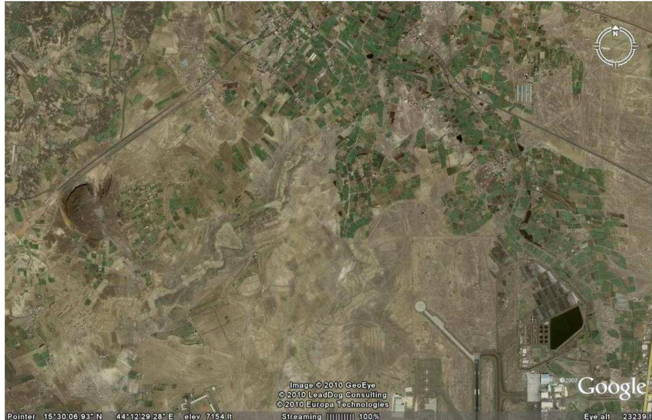
This photograph shows a good example of wastewater reuse in Yemen. The treatment plant (right below) is the source for irrigation water. The effluent is discharged in a little wadi, where it is pumped to the various fields along the stream.
