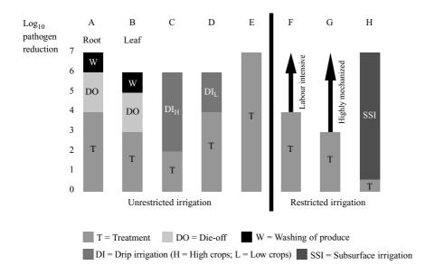
Figure 4: Examples of Options for the Reduction of Pathogens by Using the "Multiplebarrier Approach"
